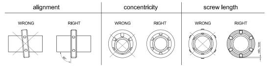
Now carefully screw the grip <u>counter-clockwise</u> onto the clamping ring.
